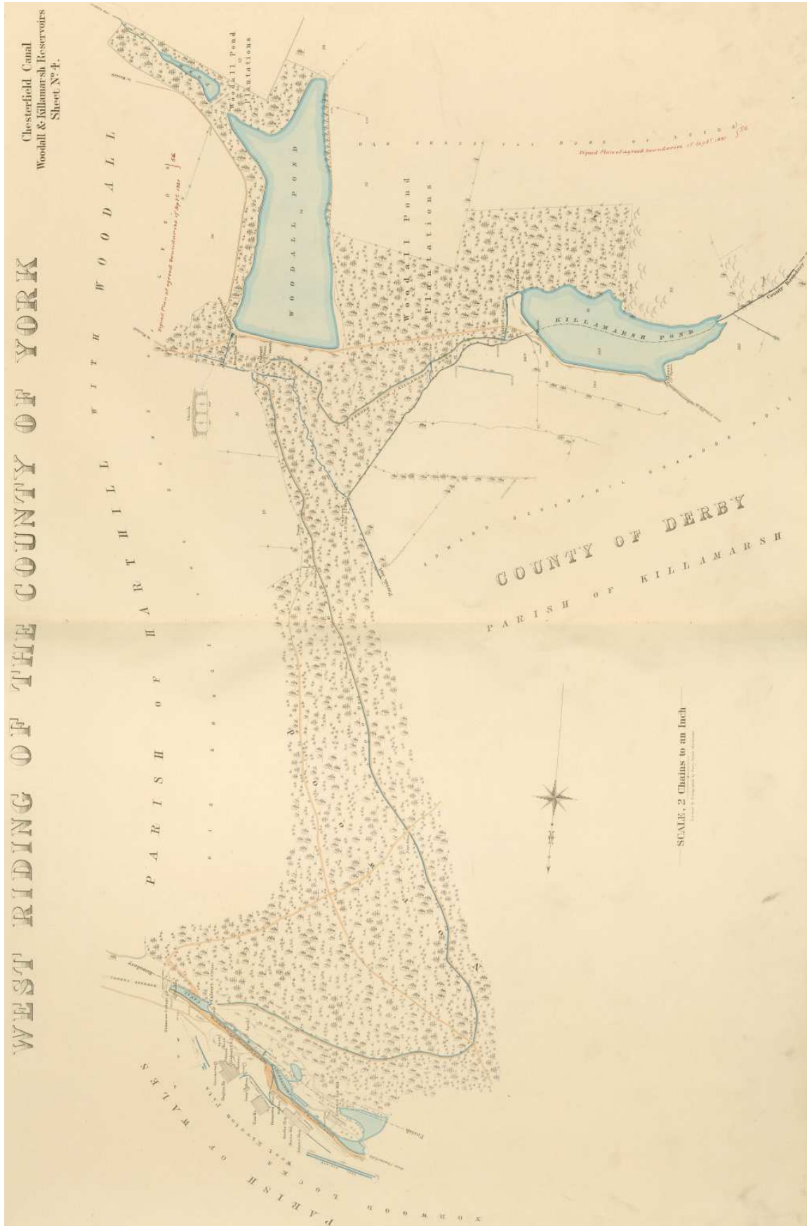
The Norwood Canal Feeder and the Woodall and Killamarsh Ponds (reservoirs) circa 1892. Taken from the Fowler Survey for the Manchester Sheffield and Lincolnshire Railway prepared at about the same time as the Derbyshire Lines were being constructed (it shows both pre and post diversion routes). The maps are dated 1892 but were probably surveyed in 1890/91).
